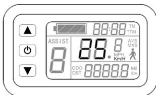
After power on for 5 seconds, hold and button at the same time, maximum riding speed KM/H flash, hold or button shortly to set the maximum riding speed (default 25KM/H). Hold button shortly and go to the next parameter settings.
