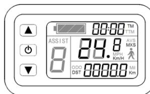
In the display of total trip time and distance, hold or button shortly to display of single maximum speed (MXS) and average speed (AVS). hold button shortly again to return the display interface. In the riding condition, 5 seconds later, automatically returns to display interface.
