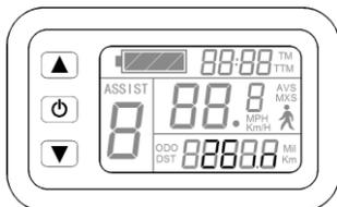
The wheel diameter will be set after finishing setting the maximum riding speed, wheel diameter specifications flashes. Hold or button shortly to set the specifications of wheel diameter. Select the range 8,10,12,14,16,18,20,22,24,26,
