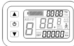
After power on for 5 seconds, hold and button at the same time, single trip riding time (TM) and single trip distance (DST) flash, hold button shortly, the content of both is cleared. If failed holding the button within 5 seconds, it will automatically return the display interface after 5 seconds, original content is preserved.
