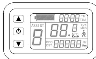
The metric units will be set after finishing setting wheel diameter, KM/H and Km or MPH and Mil flash. Hold or button shortly and select the metric units of speed and mileage in synchronization.
