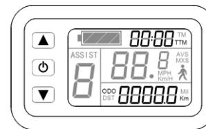
Hold button shortly to display of total trip time (TTM) and total trip distance (ODO). hold button shortly again to return the display interface. In the riding mode after 5 seconds, automatically returns to display interface.
