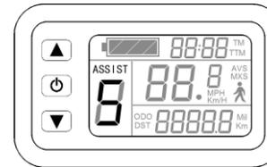
Hold or button shortly to switch 1-5 file gear. Gear 1 is for the minimum power, gear 5 is for the highest power. Each startup will automatically restore the gear shutdown last time. Gear 0 is without booster function.
