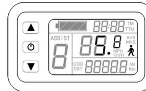
Hold button and flashes, the vehicle drives at the speed not more than 6Km/h. Release button, the function is invalid.
